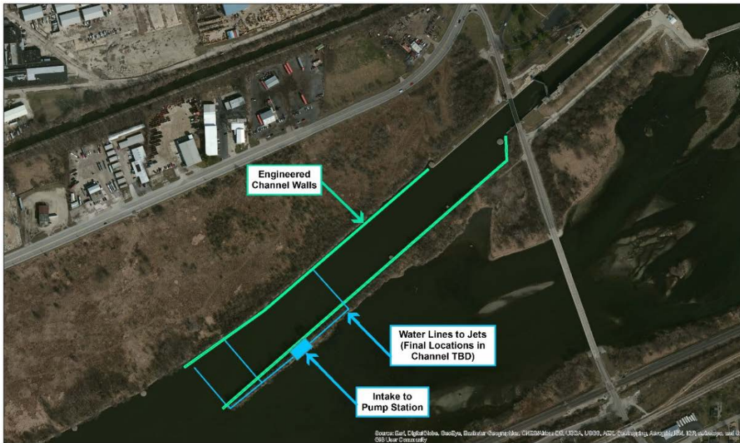
Figure 6-8 Conceptual Layout of Water Jet System in BR Downstream Approach Channel
