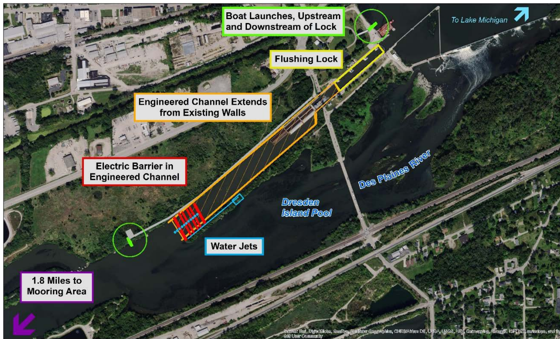
Figure 6-31 Aerial View of BRLD with Technology Alternative – Electric Barrier
