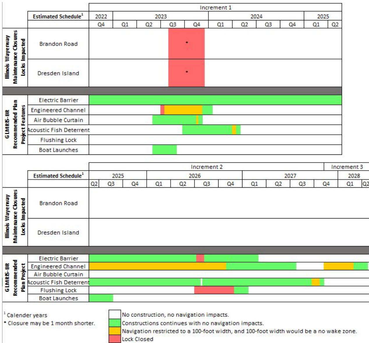
Figure S-1 Illinois Waterway Maintenance Closures, Estimated Construction Schedule for the Recommended Plan with Impacts on Navigation Identified
